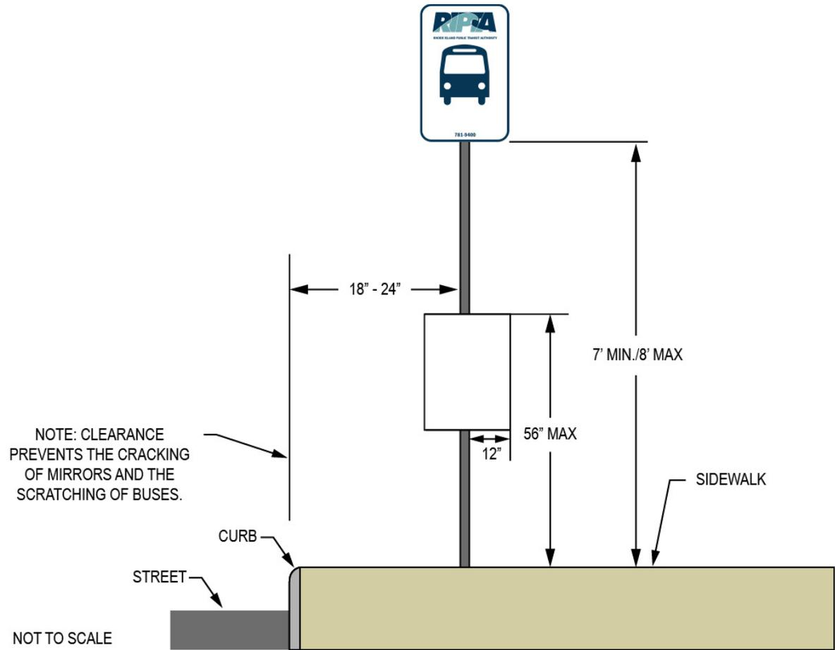
**Figure 4.3 Bus Stop Sign and Post Placement<sup>24</sup>**
