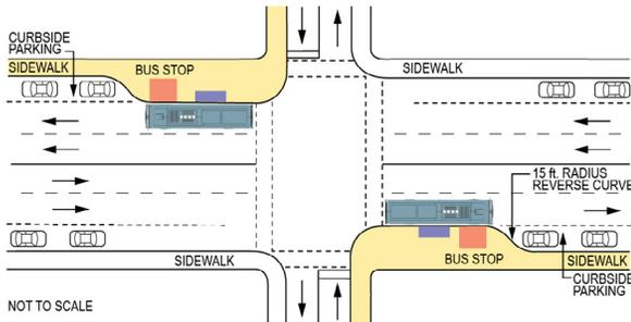
Figure 2.13 Bus Stop Curb Extension Far-side<sup>14</sup>
