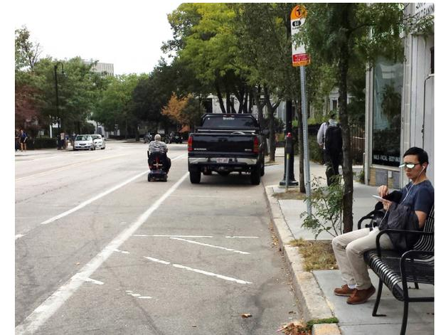
*Benches should not be positioned less than 5 feet from the curb when facing the roadway*
