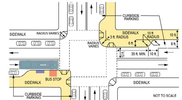
**Figure 2.12 Bus Stop Curb Extension Near-side<sup>13</sup>**
