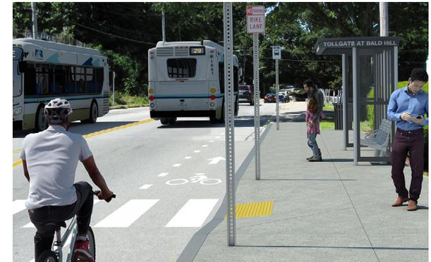
Figure 4.2 Signage at a Conceptual RIPTA Bus Stop in Bike Lane on Toll Gate Road at Bald Hill Road in Warwick, RI
