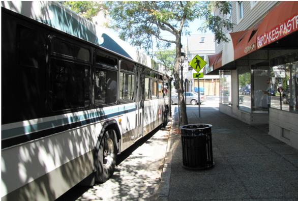
RIPTA stop on Route 114 at Child Street/Route 103 in Warren, RI has insufficient stop length to enable the bus to pull parallel to the curb
