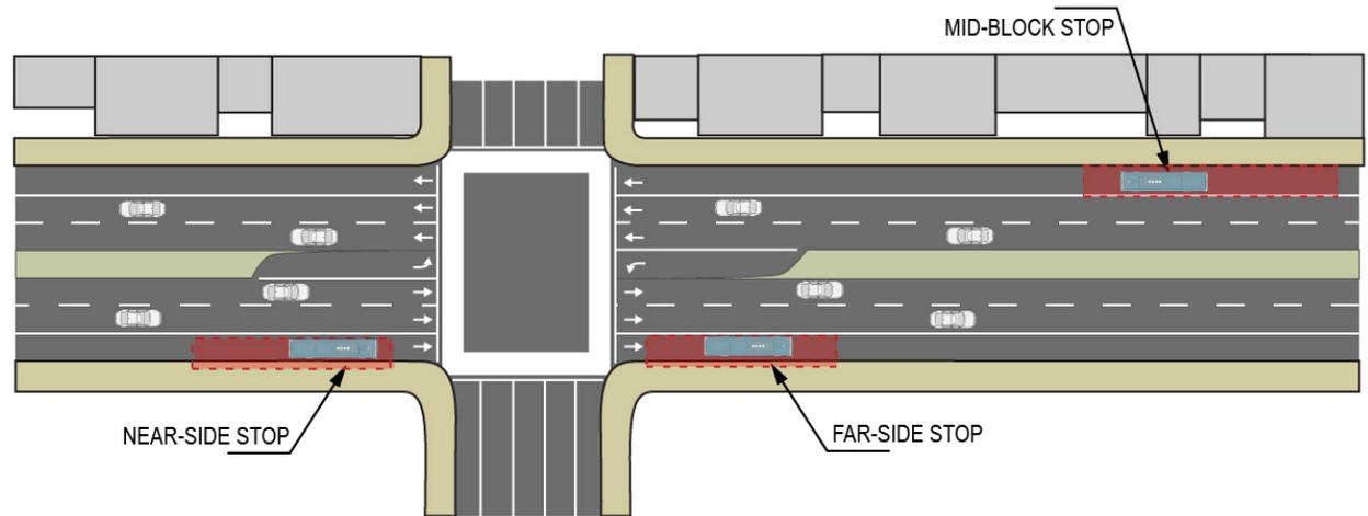
Figure 2.1 Far-side, Near-side and Mid-block Located Bus Stops<sup>2</sup>
