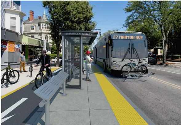
**Figure 5.6 Conceptual RIPTA Floating Bus Stop on Broadway at Knight Street in Providence, RI**
