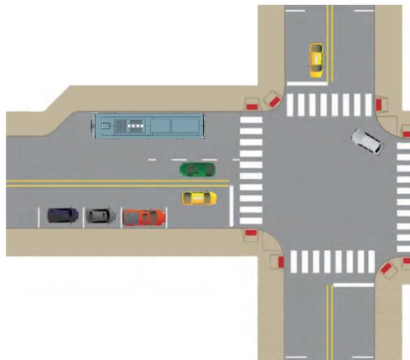
Figure 2.7 Far-side Open Bus Stop Pull Out<sup>5</sup>
