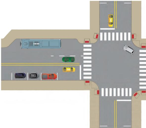
Figure 2.8 Far-side Partial Open Bus Stop Pull Out<sup>7</sup>
