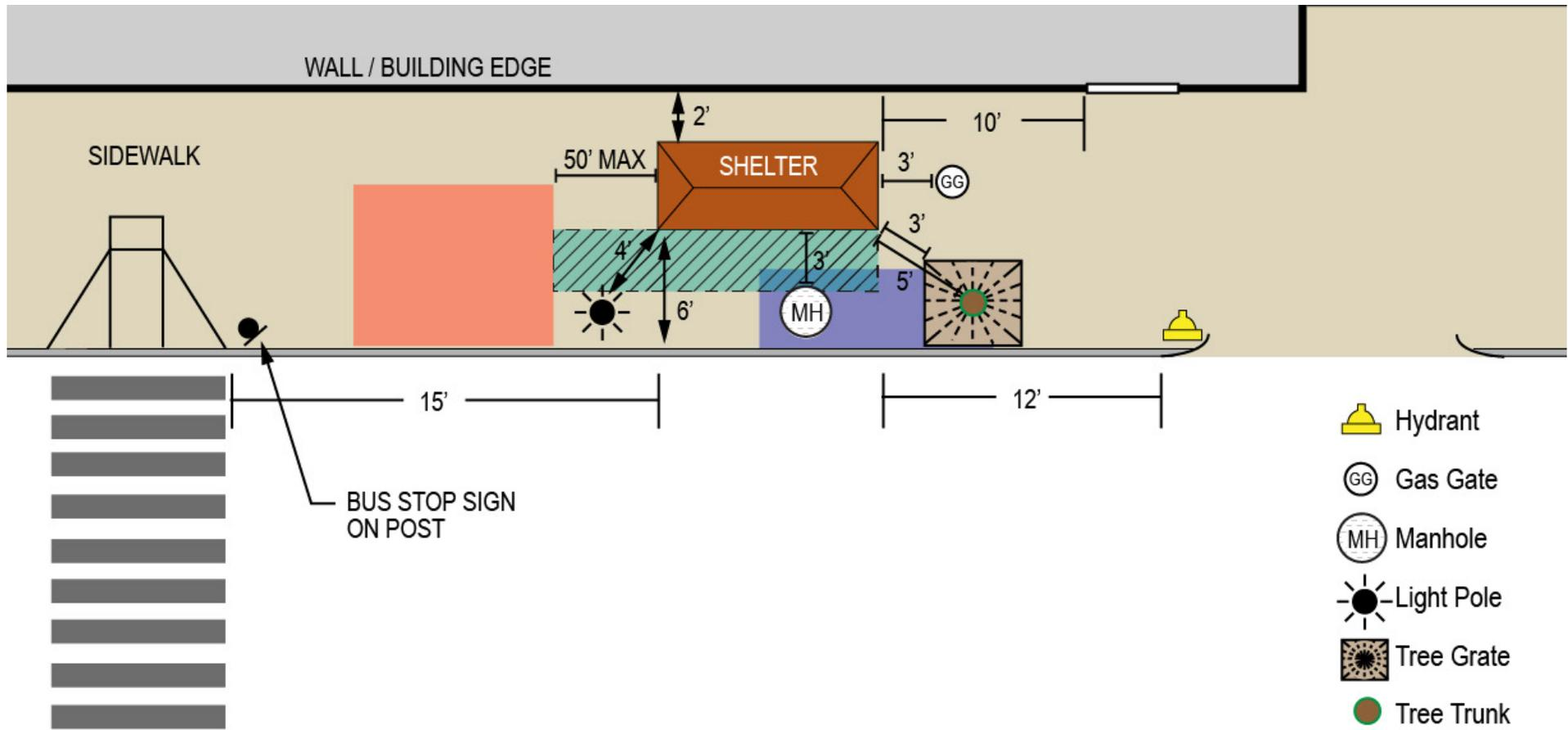
Figure 6.3 Detailed Shelter Clearances<sup>30</sup>
