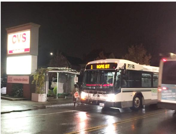
*RIPTA stop on Hope Street at Lauriston Street in Providence, RI has a curb extension to the rear of the stop, prohibiting the bus operator from pulling to the curb, forcing them to discharge passengers in the roadway rather than onto the sidewalk*
