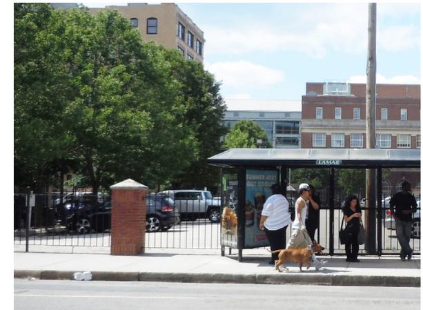
though the ADA requires a minimum 3-foot wide path. Although not desirable, the width may be reduced at pinch points, for example at a utility pole, to 3 feet, as long as the other clearances are met. The ADA guidelines allow for a minimum 32 inches; however, this should not be permitted without exceptional, extenuating circumstances. To the extent feasible this accessible path of travel should be provided to other bus stop amenities as well.
