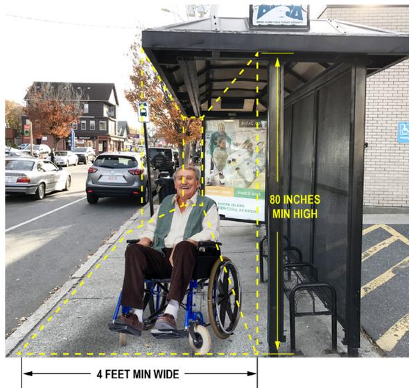
**Figure 3.4 Pedestrian Vertical and Horizontal Clearances<sup>22</sup>**
