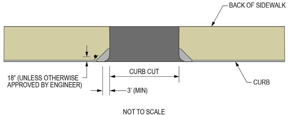
**Figure 4.4 Bus Stop Sign Placement at Driveway**
