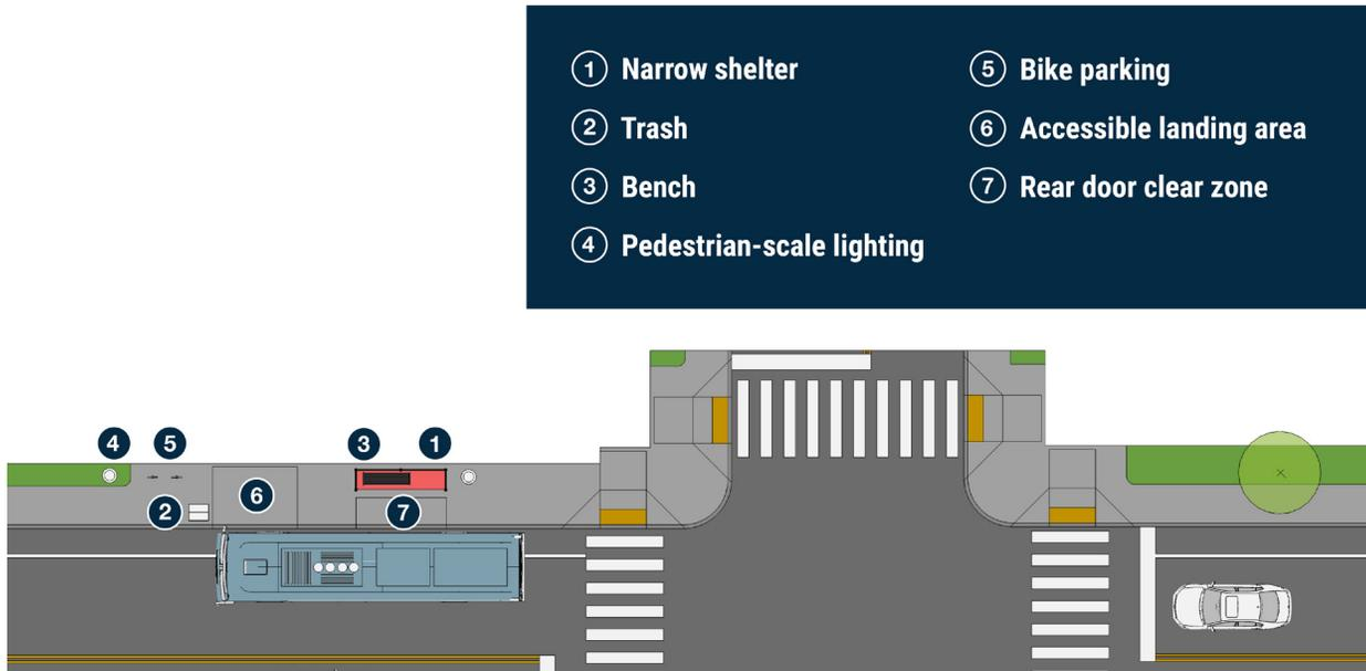
**Figure 4.5 Pedestrian-scale Lighting at a Bus Stop**
